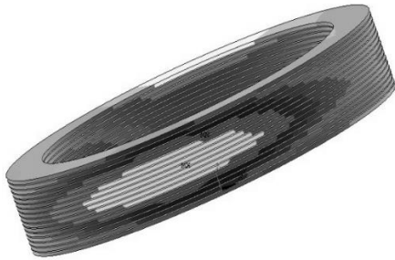
Figure 5: Distribution of deformations on the windings.
